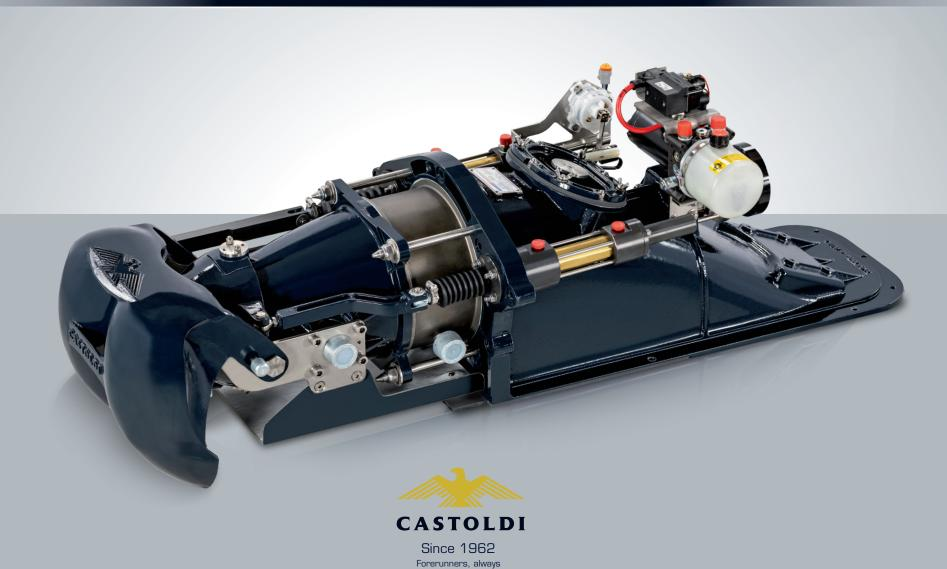
**Turbodrive 224 D.D.** is the only model of the range not equipped with the integrated gearbox but directly matched to the engine through the impeller, presently designed to match engines with 110 mHP @ 3.200 rpm or others with power and rpm lying on the same cubic curve.
